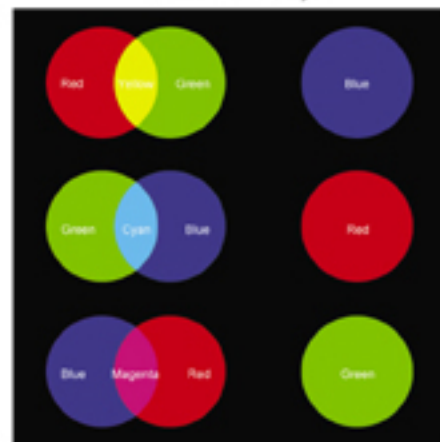
Figure 1-21. The primary spectral colors follow the principle of additive color when combined in equal amounts to make the secondary colors (left) of the human visual spectral system. The secondary spectral colors are deficient one primary spectral color, which is their complementary color (right) and recombines in equal ratios as white light.
