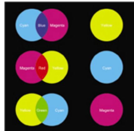
Figure 1-23. The primary pigment colors follow the principle of subtractive color mixing (when combined in equal amounts) to make secondary color pigments (left). These secondary color pigments lack one primary pigment color, which is their complementary color (right) and, mixed in a certain ratio, produce black.
