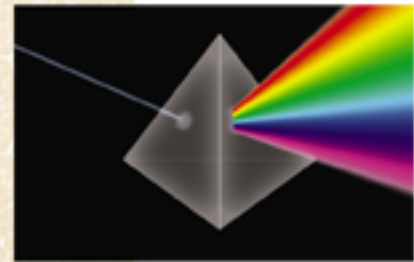
Figure 1-1. Newton's experiment in atmospheric optics demonstrates the decomposition of a ray of white light into rays of different colors by means of a glass prism.
